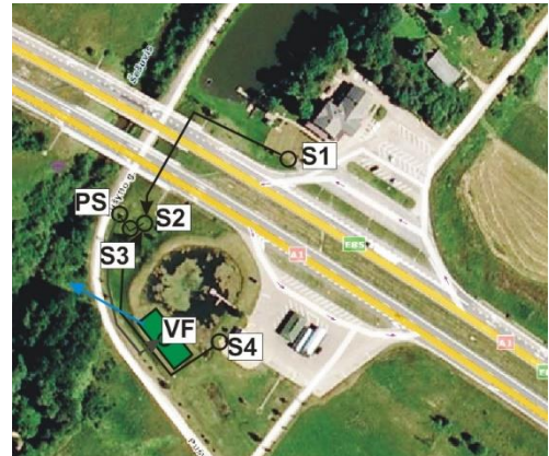
S1...S4 – septic tanks; PS – pump shaft; VF – sub-surface vertical flow constructed wetland
