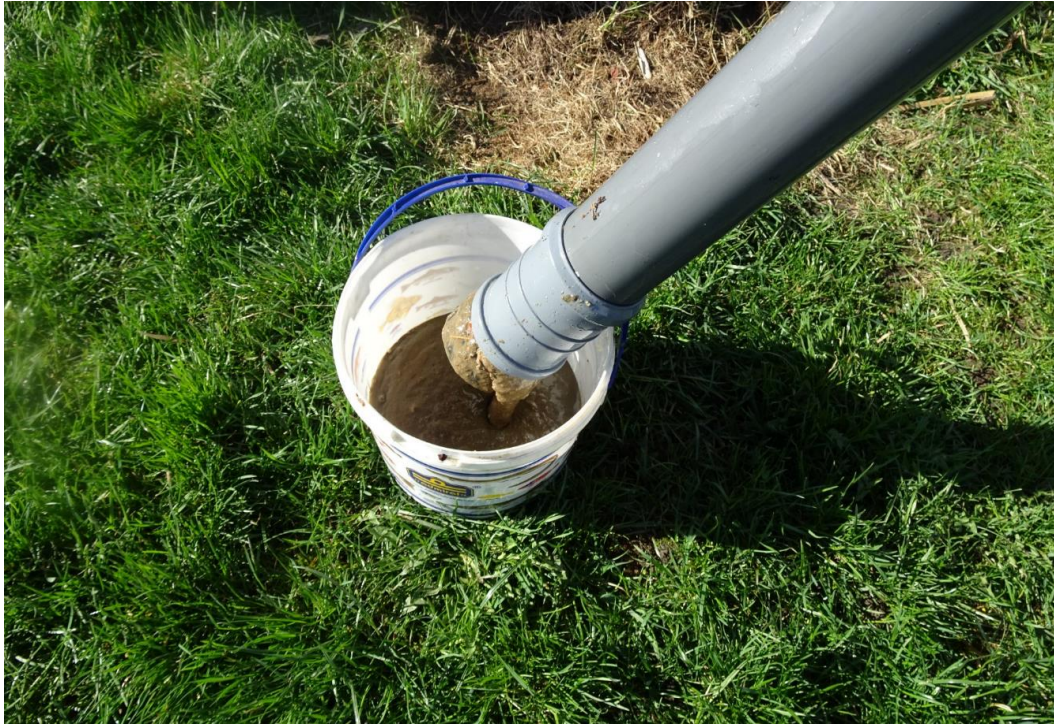
Figure 3.5.1.6. The sludge taken from the sedimentation tank [own photo, 04.2017]
